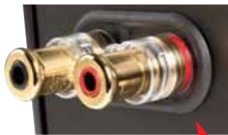
The high-quality WBT jacks are mounted on special rubber "impact sound interrupters"
