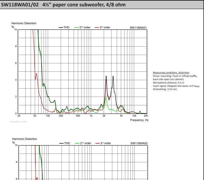
Measuring conditions, distortion Driver mounting: Flush in infinite baffle, back side open (no cabinet) Microphone distance: 0.5 m Input signal: Stepped sine wave, 5.7 V<sub>RMS</sub> Smoothing: 1/12 oct.
