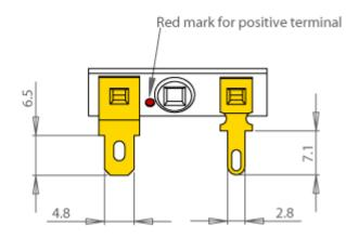
Thickness, both terminals: 0.5mm Terminal plating: Gold
