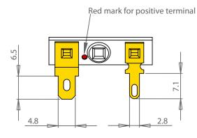
Thickness, both terminals: 0.5mm Terminal plating: Gold
