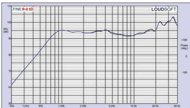
Figure 6: Wavecor TW045WA01 two-sample SPL comparison
