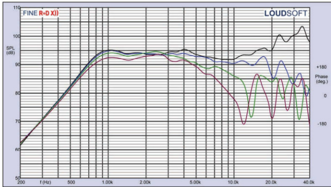
Figure 3: Wavecor TW045WA01 horizontal on- and off-axis frequency response (0°=black; 15°=blue; 30°=green; 45°=purple)
