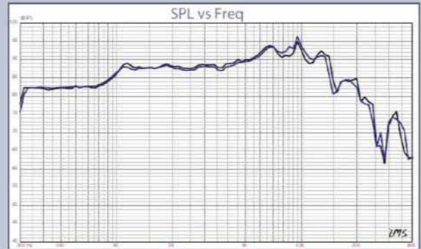
FIGURE 29: Wavecor WF120BD04 two-sample SPL comparison.
