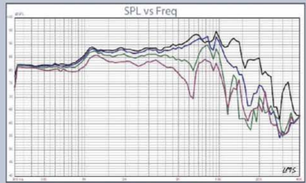
FIGURE 28: Wavecor WF120BD04 on- and off-axis frequency response.
