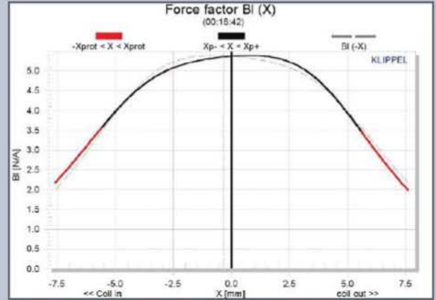
FIGURE 22: Klippel Analyzer BI (X) curve for the Wavecor WF120BD04.
